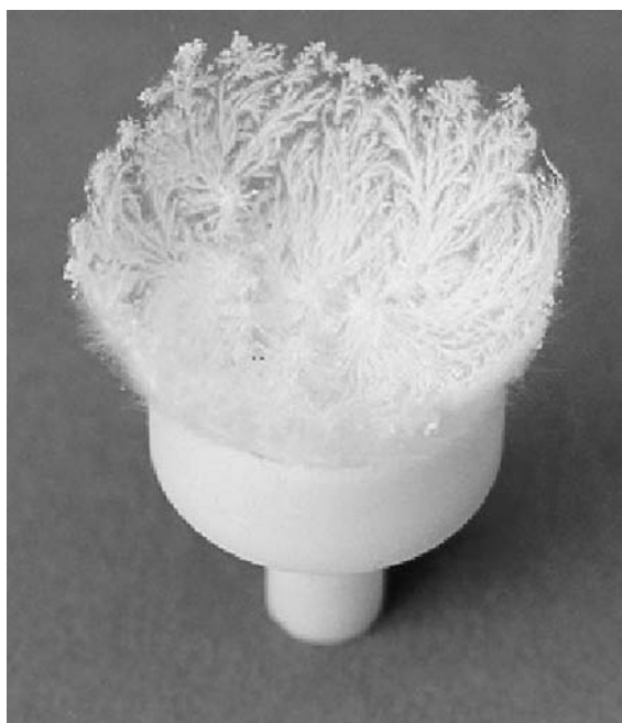
Fig. 10. Photo of the ZnO sample after an interrupted dissociation experiment in air.
