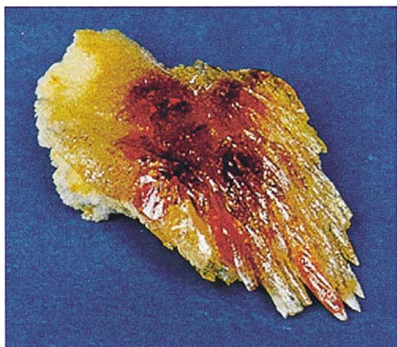
Fig. 5. Photo of a red ZnO crystal (3 cm in diameter) with excess zinc in its lattice, obtained by solar heating in air, followed by fast cooling.
